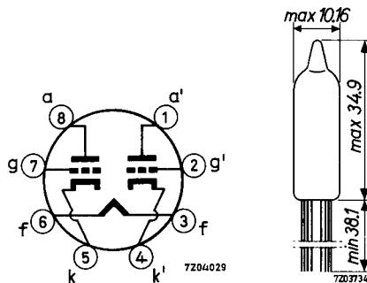
The leads should not be soldered nearer than 5 mm to the seal and should not be bent nearer than 1.5 mm to the seal.
